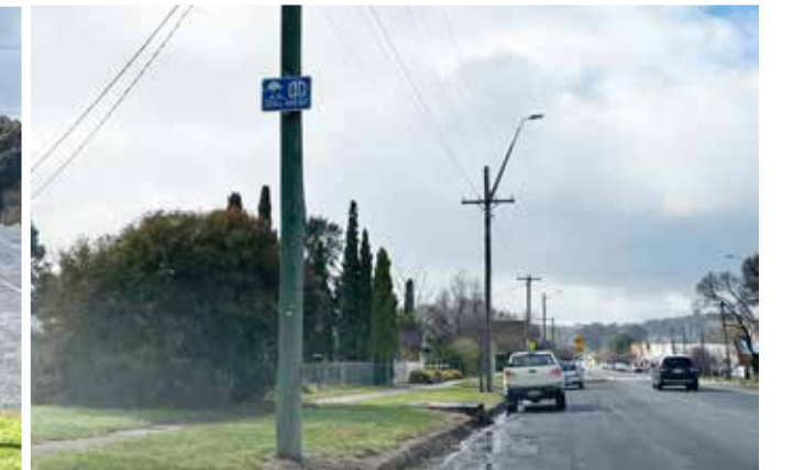
Gunning - ineffective undersized sign 3m off the ground
