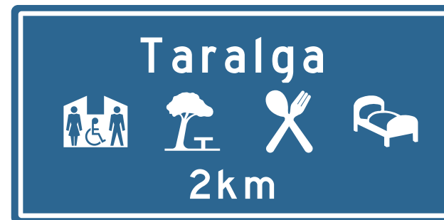
EXAMPLE -Blue Visitor Services advance warning sign
