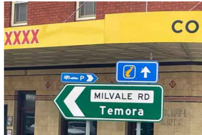
Young - Road name and green directional signage should always be positioned at the top of the signage stack, all other signed below
