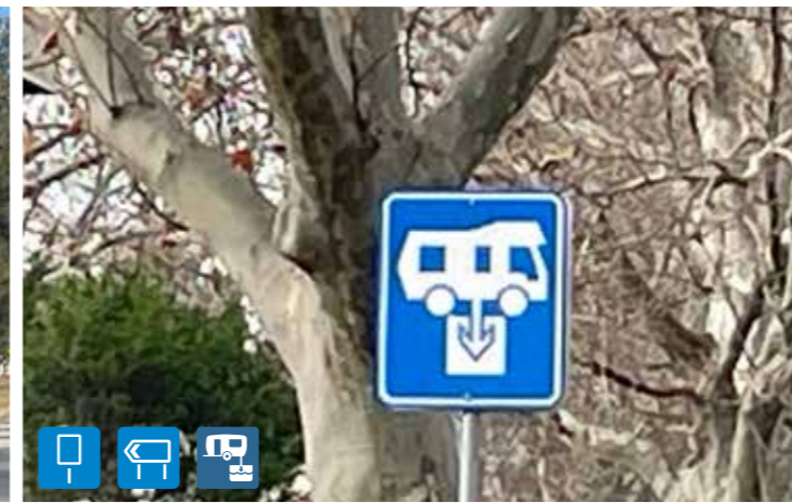
Yass RV Dump point - This location has visibility issues, advance warning signs should be positioned 200m either side of this location with a double sided directional sign opposite the entrance to the car park (see example page 37)
