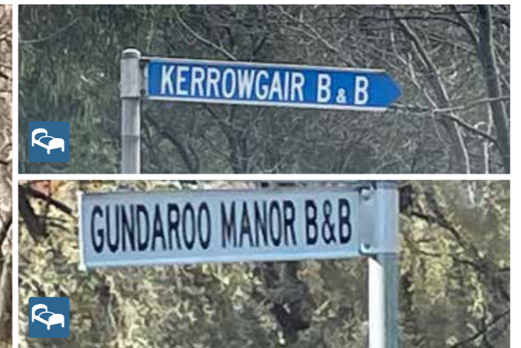
Accommodation signs should be white text on a blue background with the Australian Standard symbols
