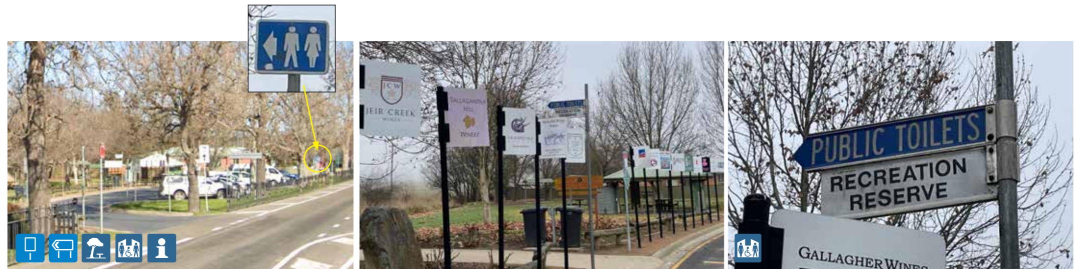
Murrumbateman Jones Park Rest Area - No advance warning or directional signage to this facility from either northern or southern approach on Barton Hwy. The only directional sign present is a symbol sign (wrong) for the toilets positioned well past the decision point for turning into the rest area
