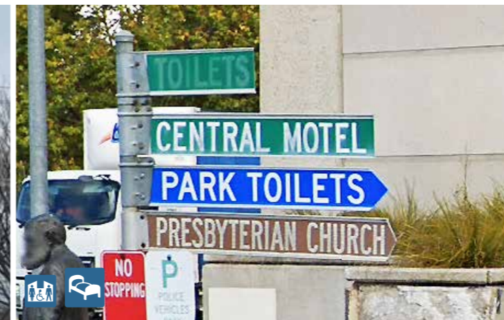
Queanbeyan - Monaro/Lowe St intersection fingerboard signs. Remove green toilets, motels should be a white on blue sign with AS accommodation symbol, Park toilets text should have AS symbol, Church is not a tourist attraction
