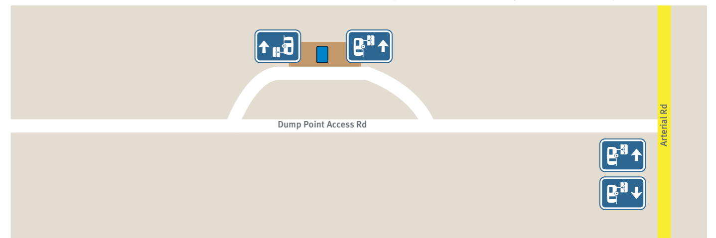
SUGGESTED - Double sided directional sign at nearest arterial road intersection with positional signs locating the dump point from both directions
